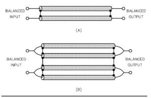
Fig 24—Shielded balanced transmission lines utilizing standard small-size coaxial cable, such as RG-58 or RG-59. These balanced lines may be routed inside metal conduit or near large metal objects without adverse effects.
